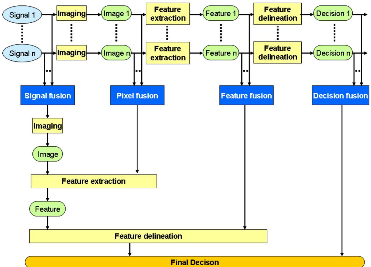
Figure 51 – Processing levels of image fusion
