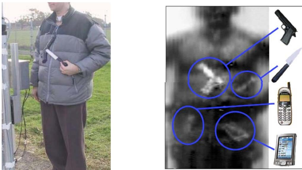
**Figure 6 – Detection of different objects**
