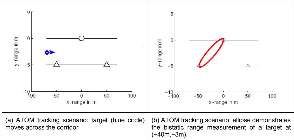
**Figure 39 – Tracking scenario: Corridor with two sources (triangles) and a single passive receiver (circle); target moving across the corridor is shown by blue circle.**
