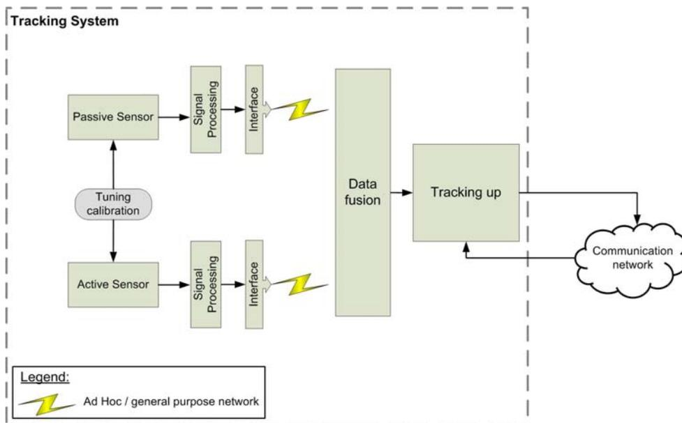
Figure 25 – ATOM Architecture: tracking system block
