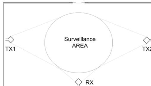
**Figure 38– Example of configuration for a Passive Radar System which exploits two transmitters of opportunity**
