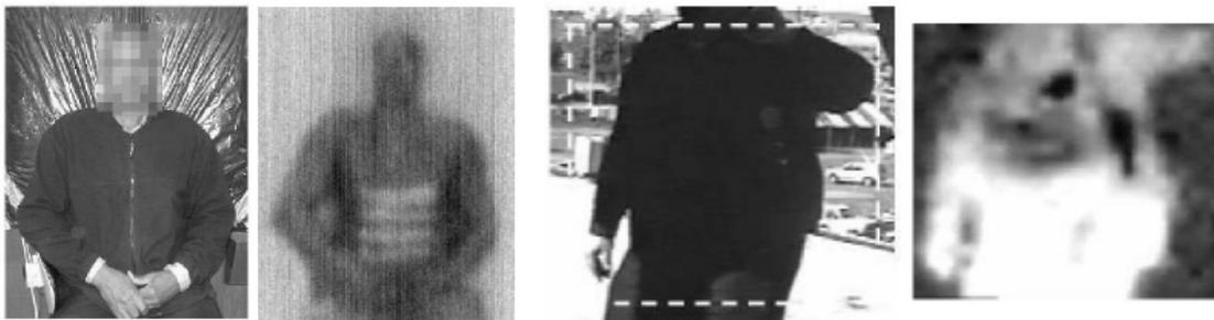
**Figure 29 – Passive mm-wave image taken (left) indoor, and (right) outdoor**
