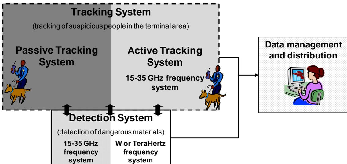
Figure 20 – Main blocks of the ATOM system
