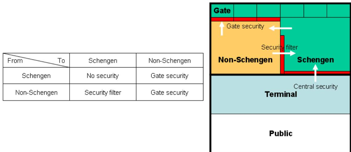
Figure 16 – Transfer passengers security concept at Schiphol airport
