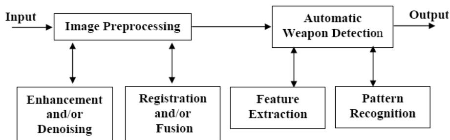
**Figure 28 – Image processing scheme for concealed weapon detection**
