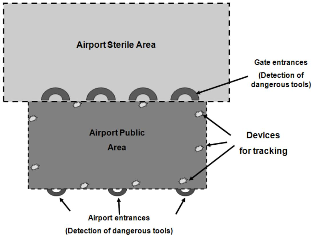
Figure 19 – Distributed controls in the ATOM system
