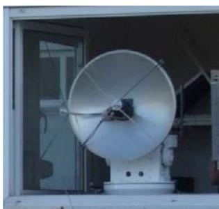
**Figure 7 – The 220 GHz radiometric system**
