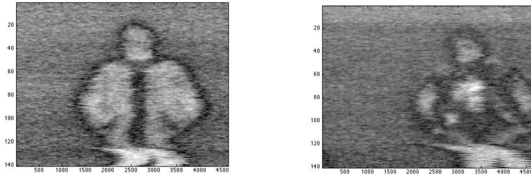
**Figure 8 – Standoff detection of the system at 220 GHz**
