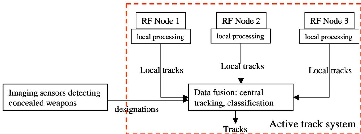
**Figure 44 – Schematic overview active tracking system**
