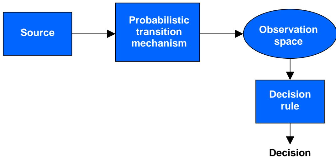
Figure 48 – Components of a hypothesis testing problem
