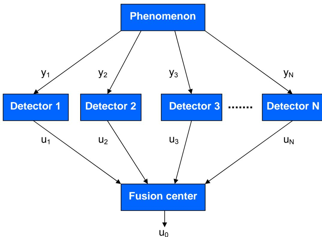
Figure 49 – Parallel fusion network
