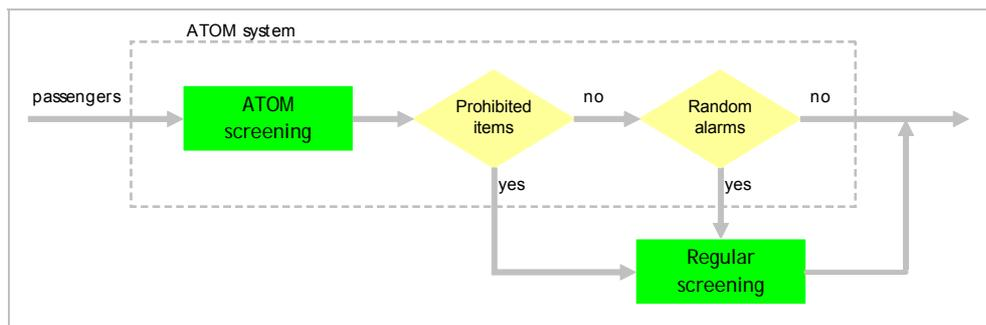
Figure 1 – Process of screening
