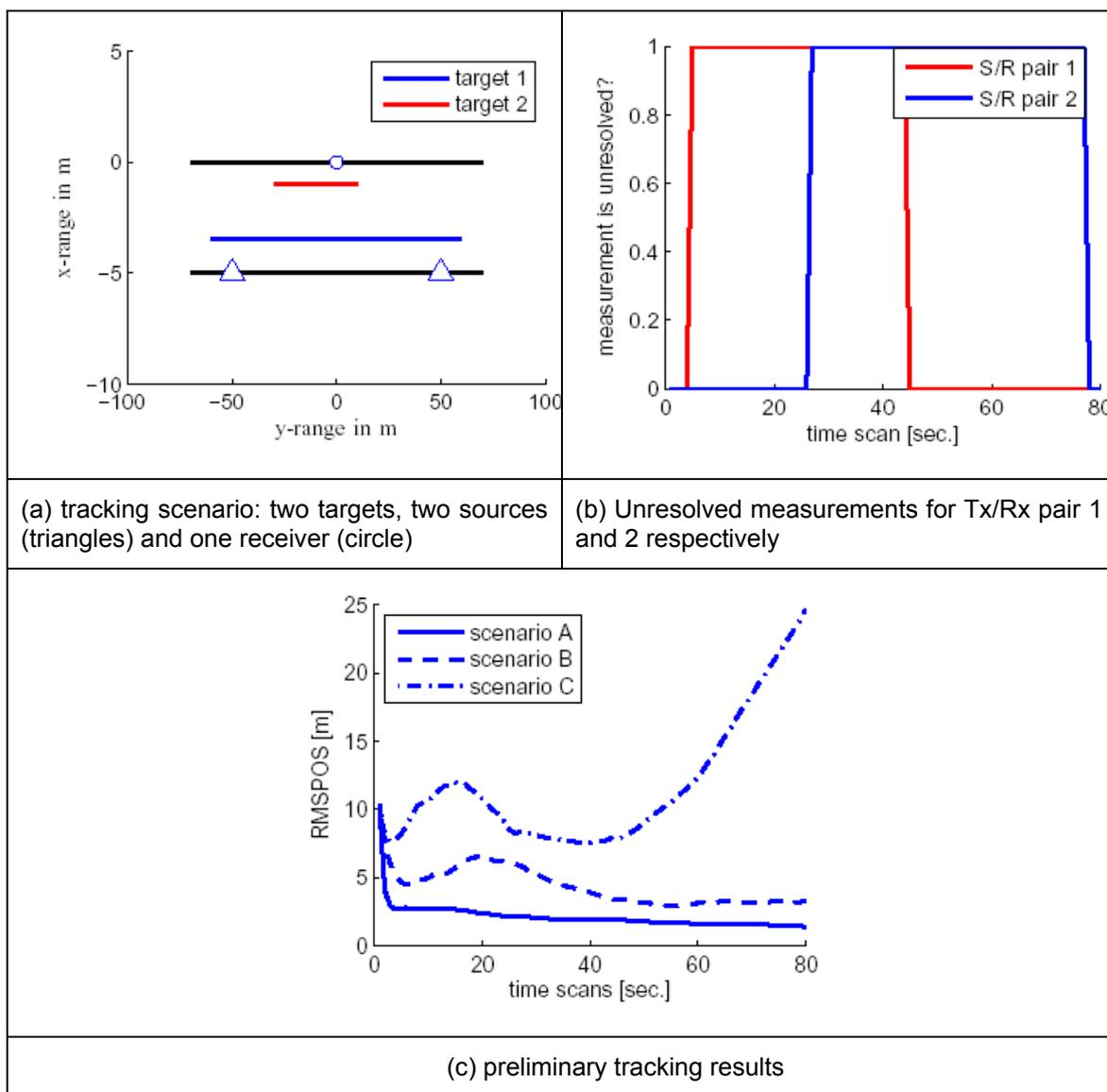
**Figure 42 – Sequential target tracking**
