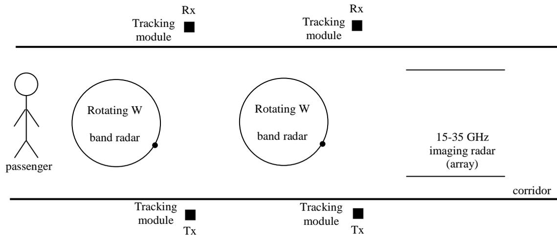
**Figure 34 – Sensor fusion of multiple imaging subsystems to determine successively the risk level of a person**
