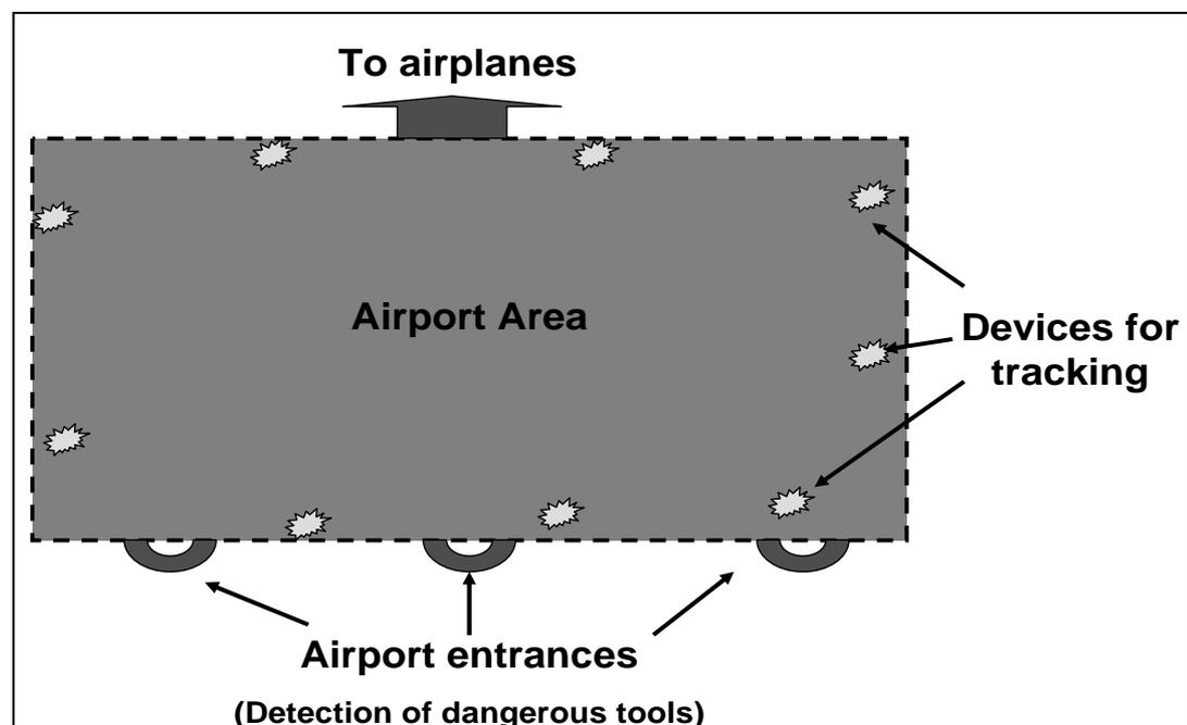
Figure 21 – Distribution of the detection and tracking sensors of ATOM system in the airport area
