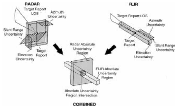
**Figure 45 – Advantage of sensor data fusion**
