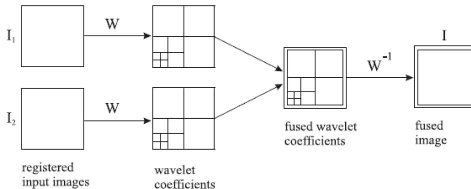
Figure 52 – Fusion of the wavelet transforms of two images
