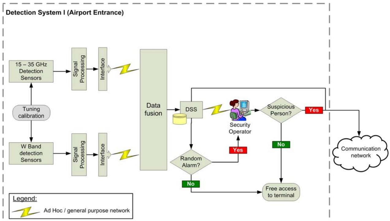
Figure 23 – ATOM Architecture: Detection system I (Airport entrance)
