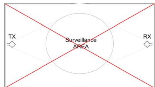
**Figure 36 – Example of configuration that must be avoided in a Passive Radar System**
