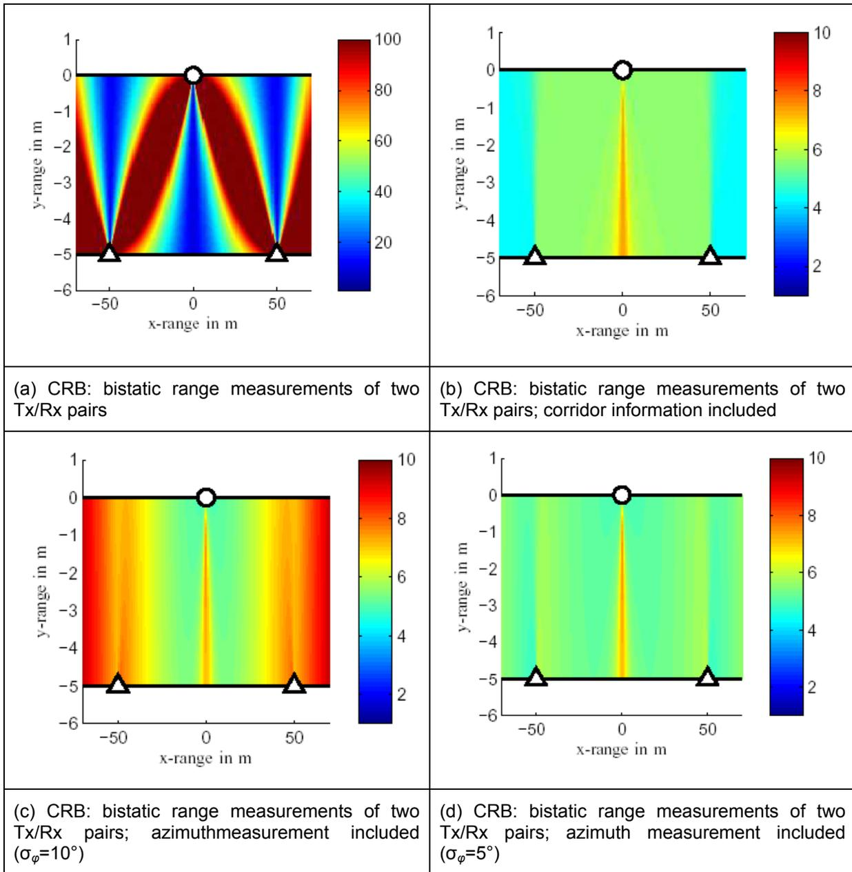
**Figure 40 – CRB of position estimate (two Tx/Rx pairs). Note the different scalings of the colorbar in (a) and (b,c,d).**
