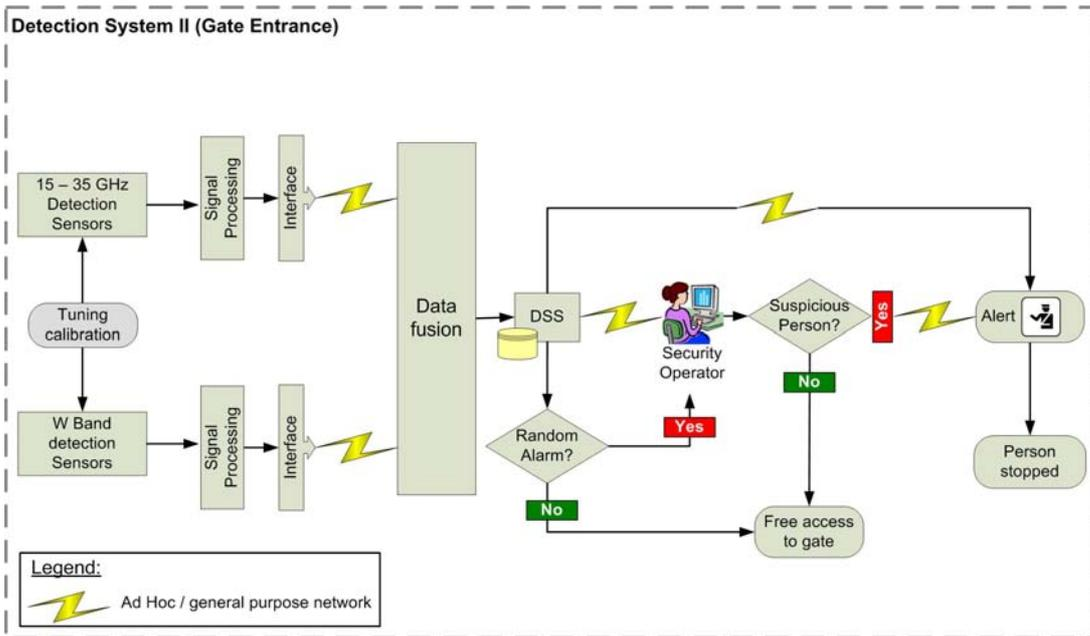
Figure 24 – ATOM Architecture: detection system II (Gate entrance)
